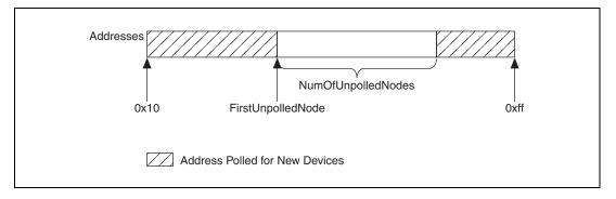
In other words, FirstUnpolledNode tells the LAS the beginning of a region of addresses to not probe, and NumOfUnpolledNodes tells the LAS the length of that region. So if FirstUnpolledNode were 0x25, and NumOfUnpolledNodes were 0xba, then no addresses from 0x25 to 0xdf would be probed. That means that if a device with an address of 0x25 were placed on this bus, the LAS would not probe it, and it would never be able to send or receive packets on the bus.
